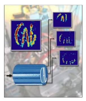
In a recent experiment the letters CAL, carved through the end of a plastic tube placed in an MRI encoding coil, were reconstructed from 10 batches of spin-polarized xenon carried to a detection coil at a separate location. Although the batches arrived at different times, the spatial arrangement of the letters was accurately reproduced.
