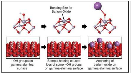
In the presence of water, aluminum ions (gray) on the surface of alumina bond to six oxygen ions (red). Heating removes the water and leaves some aluminum ions with only five oxygen ions, creating a bonding site for the barium oxide. Image courtesy of PNNL.
