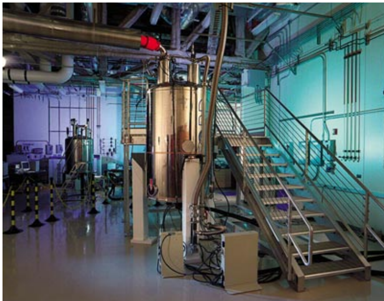
Pacific Northwest National Laboratory's NMR spectrometer
