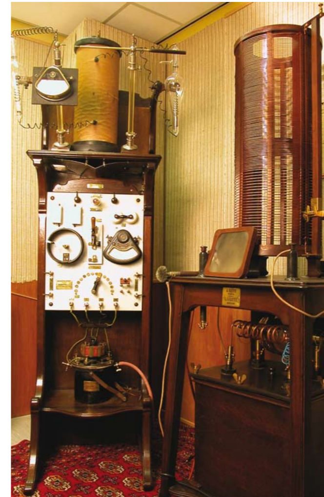
Figure 1: This widely-distributed "Art-Nouveau" model, elaborated by A.-J. D'Arsonval, (France, 1851–1940) and manufactured by G Gaiffe (France 1857–1943) enjoyed an excellent reputation and over the years underwent a number of improvements. Here, it is shown with the famous Rochefort high voltage coil at the top of the device supplied by alternating current through a mercury and gas atmosphere turbine at the bottom.
