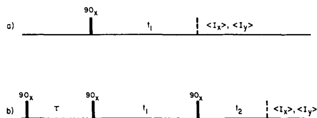
Figure 2. Simple pulse sequences for NMR experiments. The sequence in Figure 2a prepares and detects only single-quantum transitions. The sequence in Figure 2b prepares and detects multiple-quantum transitions.
