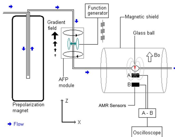
**Fig. 1.** Experimental setup. Water is prepolarized by flowing it through the magnet. The magnetization is periodically inverted by passing the liquid through the adiabatic fast passage (AFP) module and is detected with a gradiometer consisting of two AMR sensors.
