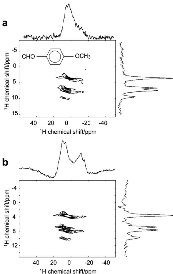
**FIG. 3.** Two-dimensional spectra of *p*-anisaldehyde in a magnetic field gradient of 0.25 mT/cm obtained using the pulse sequences displayed in Figs. 1a (a) and 1b (b). Both spectra were acquired with immediate detection after the pulse(s) and a shearing transformation corresponding to a ratio  $k = t_1/\tau = 6.2$ . The nominal  $90^\circ$  pulse length in (b) was 10  $\mu\text{s}$ .
