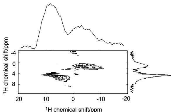
FIG. 5. Depth-sensitive  $^1\text{H}$  NMR spectrum of the samples displayed in Fig. 4a, obtained with the pulse sequence of Fig. 1a in a field gradient of 0.18 mT/cm. The spectrum was acquired with immediate detection after the pulse and a shearing transformation corresponding to  $k = t_1/\tau = 7.0$ .
