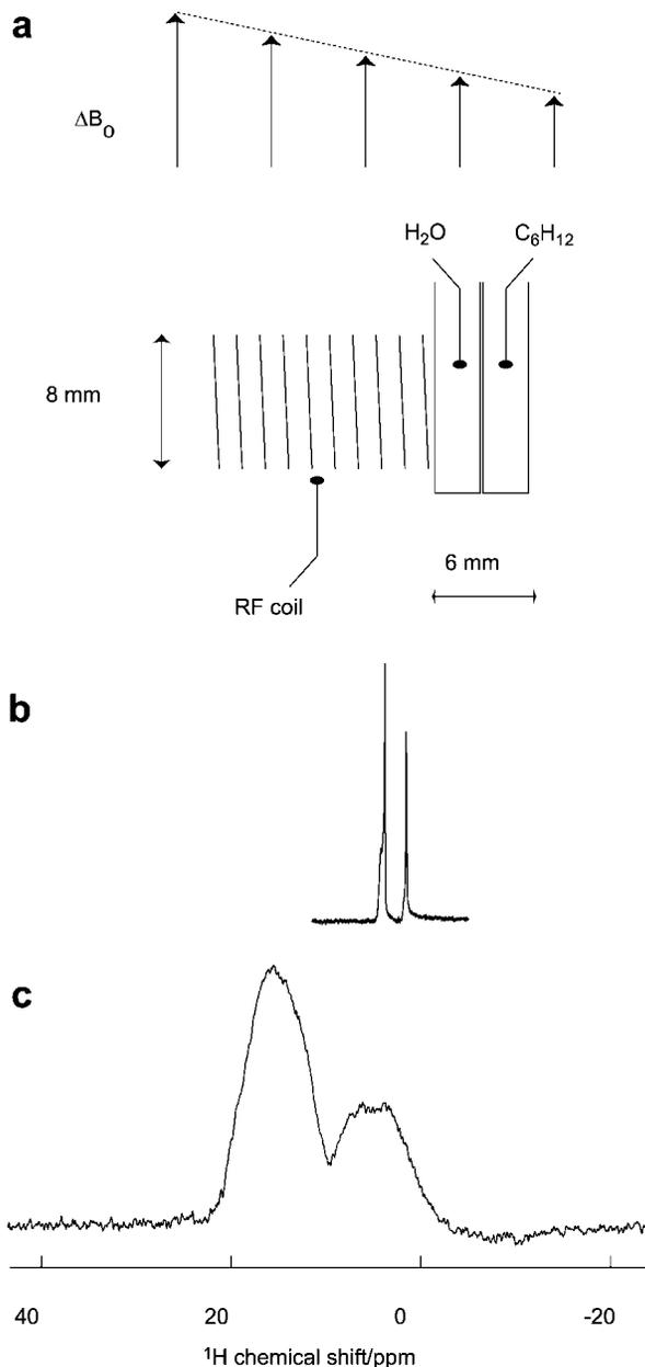
**FIG. 4.** (a) Sample setup with two tubes containing water and cyclohexane. (b) Homogeneous NMR spectrum obtained after one single pulse of length 14  $\mu\text{s}$ . (c) Inhomogeneously broadened one-pulse spectrum in the presence of a constant gradient of 0.18 mT/cm.
