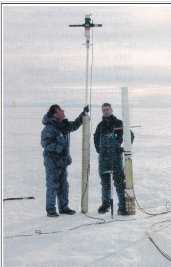
MOBILE NMR PROBE (right) developed by Paul Callaghan (holding drill at left), Mark Hunter and other researchers was dropped into a drill hole to assess the physical properties of Antarctic sea ice.
